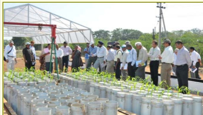
Lysimeter facility for measuring the transpiration efficiency being demonstrated and explained to visitors
